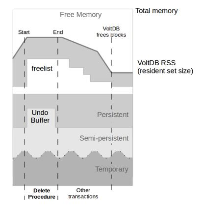
Figure 5.2. Details of Memory Usage During and After an SQL Statement
